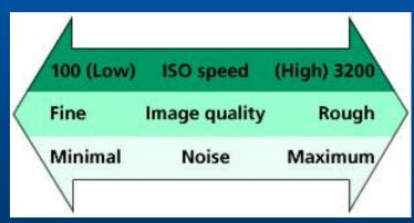
The lower the ISO speed, the finer the image grain. And the higher the ISO speed, the rougher the grain. Keep this in mind when setting the ISO speed to match the scene or lens.
